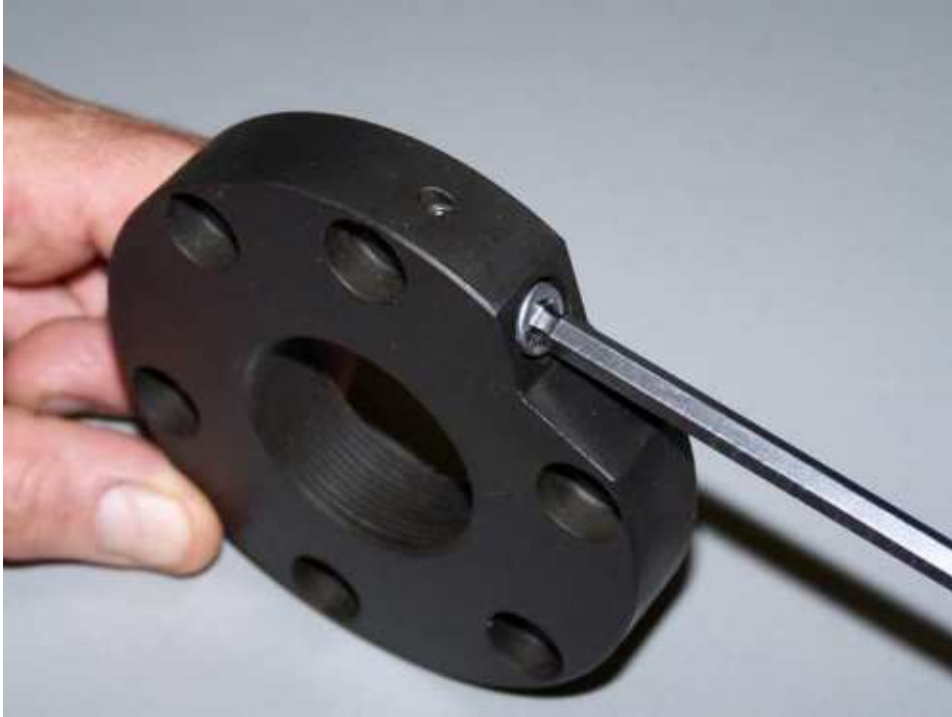
2) Loosen the flange / cylinder fixing screw
