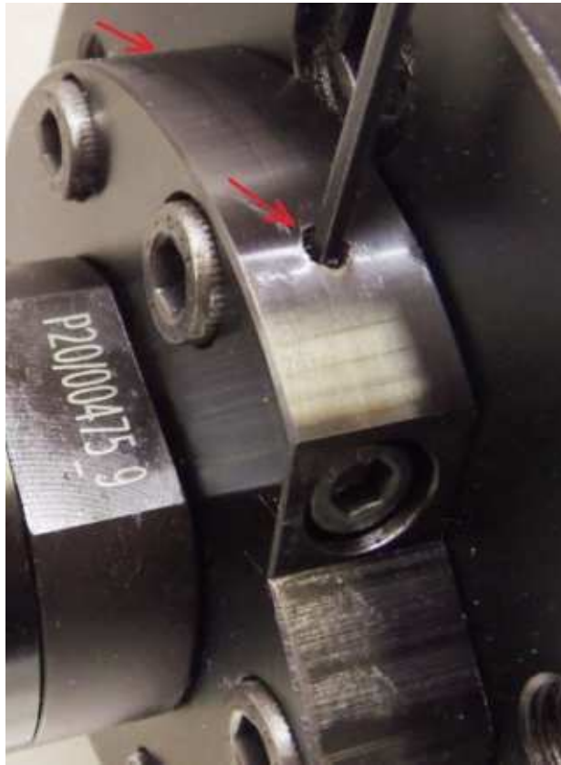
11) Loosen the grub screws behind locking bushings
