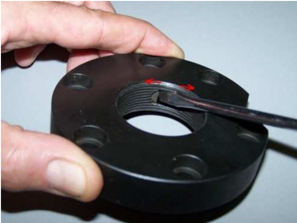
2) Loosen the flange / cylinder fixing screw
