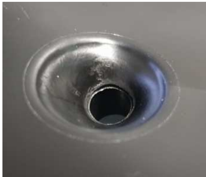
Example photo of a part injected using preload
