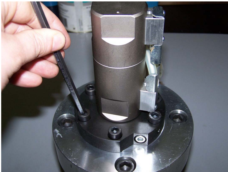
4) Fix the flange on the mould
